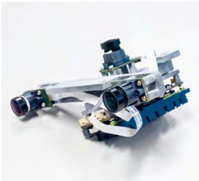
The visual-inertial sensor developed at Sevensense allows robots to see their environment and estimate their positions with respect to it.
